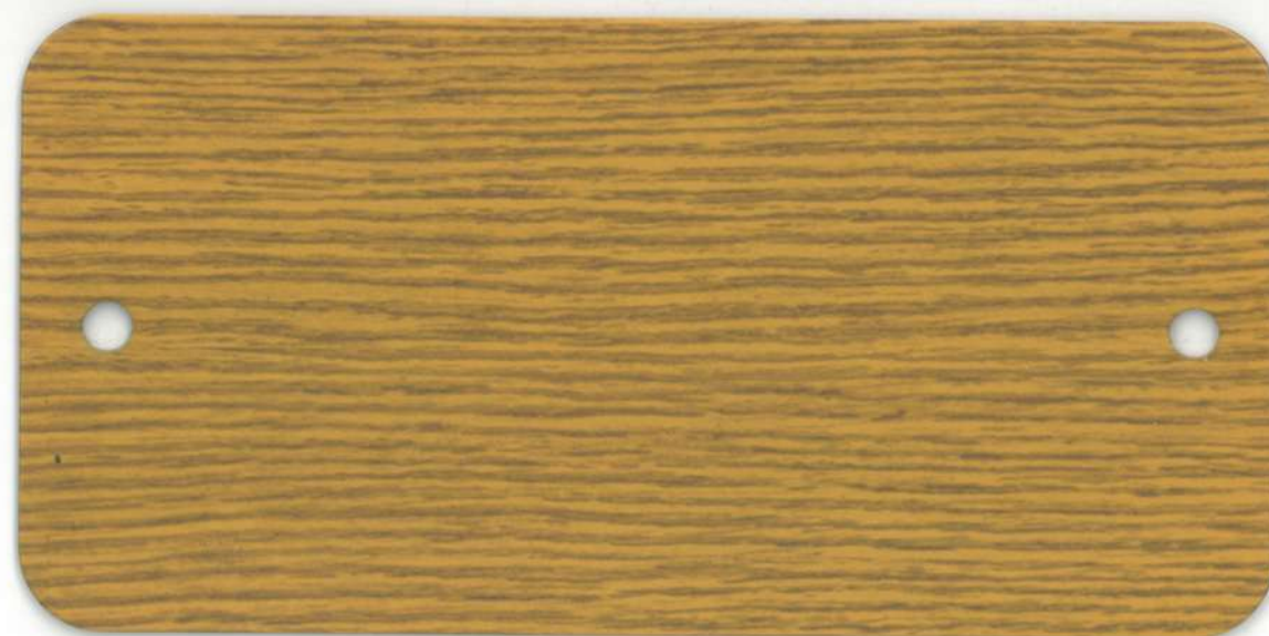
Powder Coating: DS 716 + Heat Transfer Film: 2516/10
