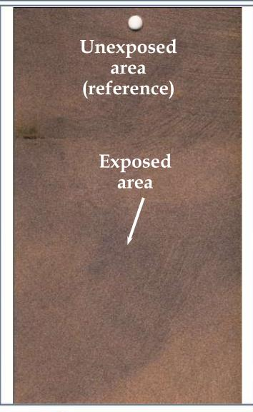
LAB. ID NUMBER: 24960 POWDER COATING: MirrorBT-022S HEAT TRANSFER FILM: 85007/01 L4 Colour variation (ΔΕ): **1,74** residual gloss: **98**%
