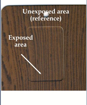
LAB. ID NUMBER: 24201 POWDER COATING: DS 772 HEAT TRANSFER FILM: -colour variation (ΔE): **0,3** residual gloss: **92%**  LAB. ID NUMBER: 24195 POWDER COATING: DS 772 HEAT TRANSFER FILM: 2531/02 colour variation (ΔΕ): **0,37** residual gloss: **90%**
