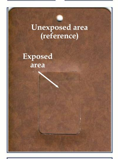
LAB. ID NUMBER: 37059 POWDER COATING: 9C-036-A004 HEAT TRANSFER FILM: 6054/01 Grey scale: 4/5 residual gloss: 80%
