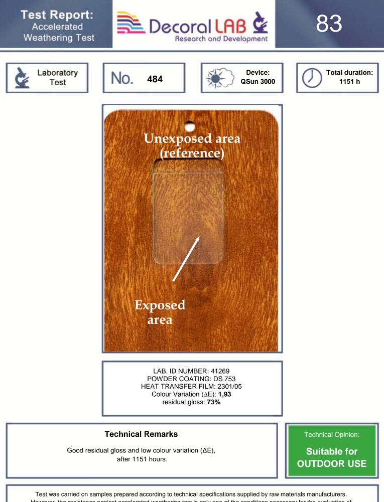
I est was carried on samples prepared according to technical specifications supplied by raw materials manufacturers.
