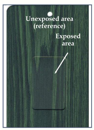
LAB. ID NUMBER: 24327 POWDER COATING: DS 747 HEAT TRANSFER FILM: -colour variation (ΔΕ): 0,12 residual gloss: 96% LAB. ID NUMBER: 24332 POWDER COATING: DS 747 HEAT TRANSFER FILM: 2503/03L colour variation (ΔΕ): **1,78** residual gloss: **89**%
