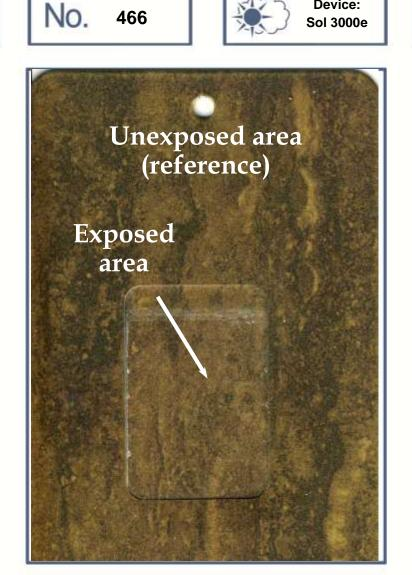
LAB. ID NUMBER: 40016 POWDER COATING: 9C-048-A004 HEAT TRANSFER FILM: 5015/08 Colour Variation ( $\Delta E$ ): 1,57 residual gloss: 90%
