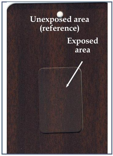
LAB. ID NUMBER: 24317 POWDER COATING: DS 742 HEAT TRANSFER FILM: -colour variation (ΔΕ): **0,11** residual gloss: **98%**  LAB. ID NUMBER: 24320 POWDER COATING: DS 742 HEAT TRANSFER FILM: 1704/02L colour variation (ΔΕ): 1,21 residual gloss: 95%
