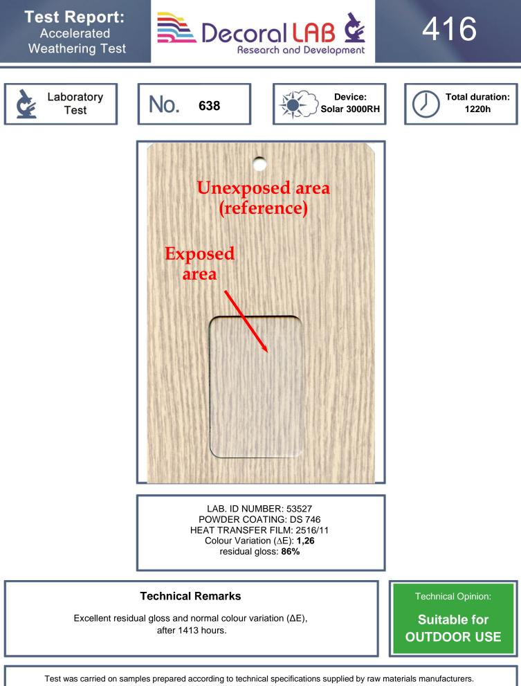
I est was carried on samples prepared according to technical specifications supplied by raw materials manufacturers. However, the resistance against accelerated weathering test is only one of the conditions necessary for the evaluation of the resistance of the finished product. For a final assessment see further analysis on natural exposure in Florida.
