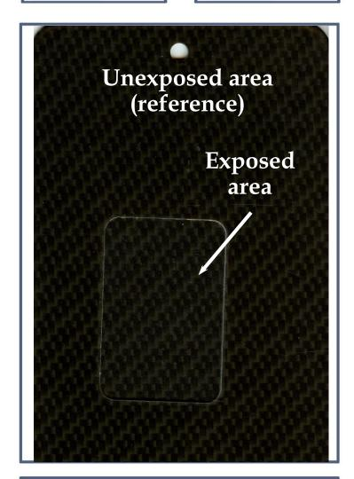
LAB. ID NUMBER: 50649 POWDER COATING: 9B-058-A004 HEAT TRANSFER FILM: 6001/01 colour variation ( $\Delta E$ ): 1,34 residual gloss: 96%
