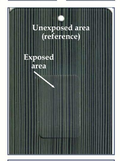
LAB. ID NUMBER: 36387 POWDER COATING: 8C-049-A001 HEAT TRANSFER FILM: 2121/02 colour variation ( $\Delta E$ ): 1,88 residual gloss: 72%
