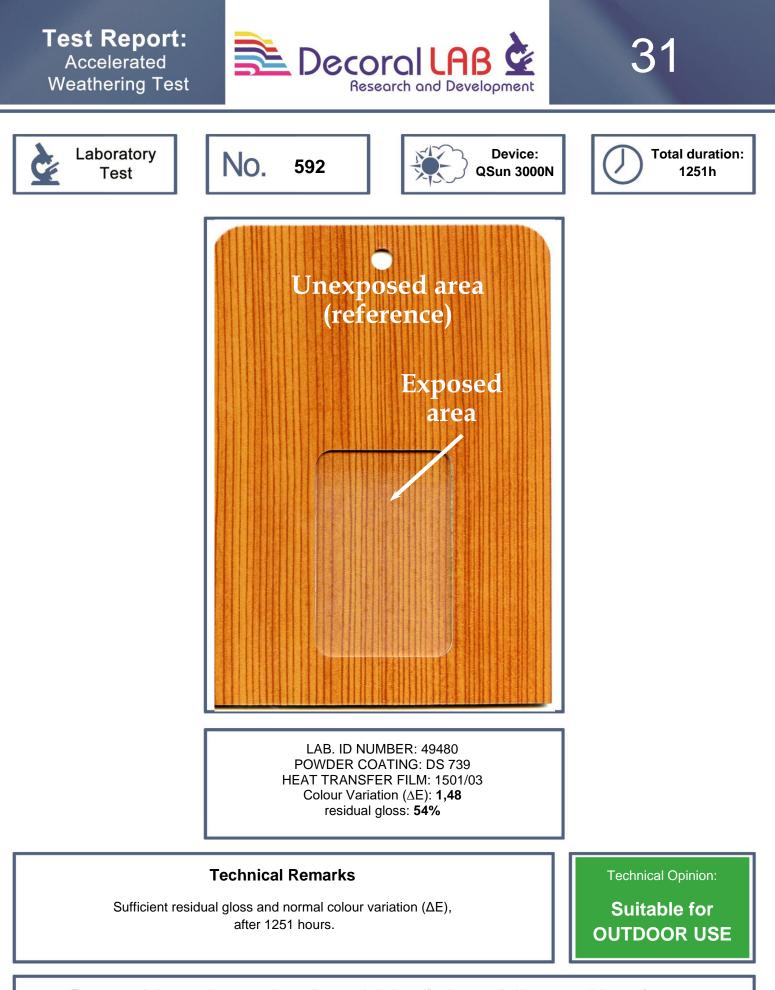
Test was carried on samples prepared according to technical specifications supplied by raw materials manufacturers. However, the resistance against accelerated weathering test is only one of the conditions necessary for the evaluation of the resistance of the finished product. For a final assessment see further analysis on natural exposure in Florida.
