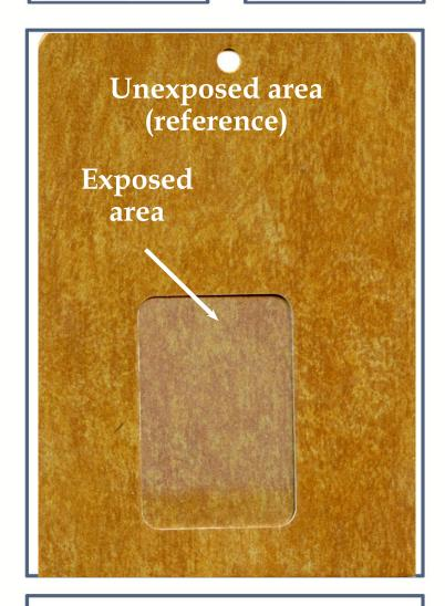
LAB. ID NUMBER: 49397 POWDER COATING: 9B-306-A050 HEAT TRANSFER FILM: 6040/06 Colour variation ( $\Delta E$ ): **5,45** residual gloss: 93%
