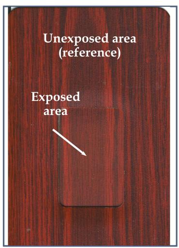
LAB. ID NUMBER: 32160 POWDER COATING: DS 794M HEAT TRANSFER FILM: -colour variation (ΔΕ): 1,55 residual gloss: 82% LAB. ID NUMBER: 32161
