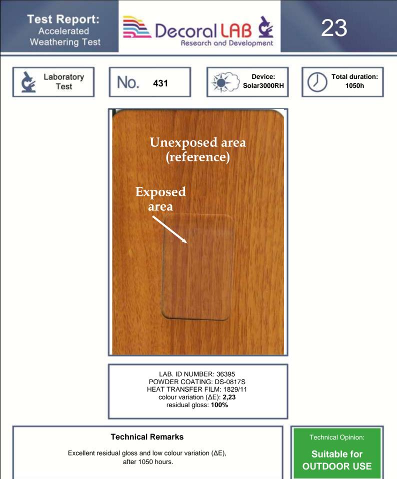
Test was carried on samples prepared according to technical specifications supplied by raw materials manufacturers.
