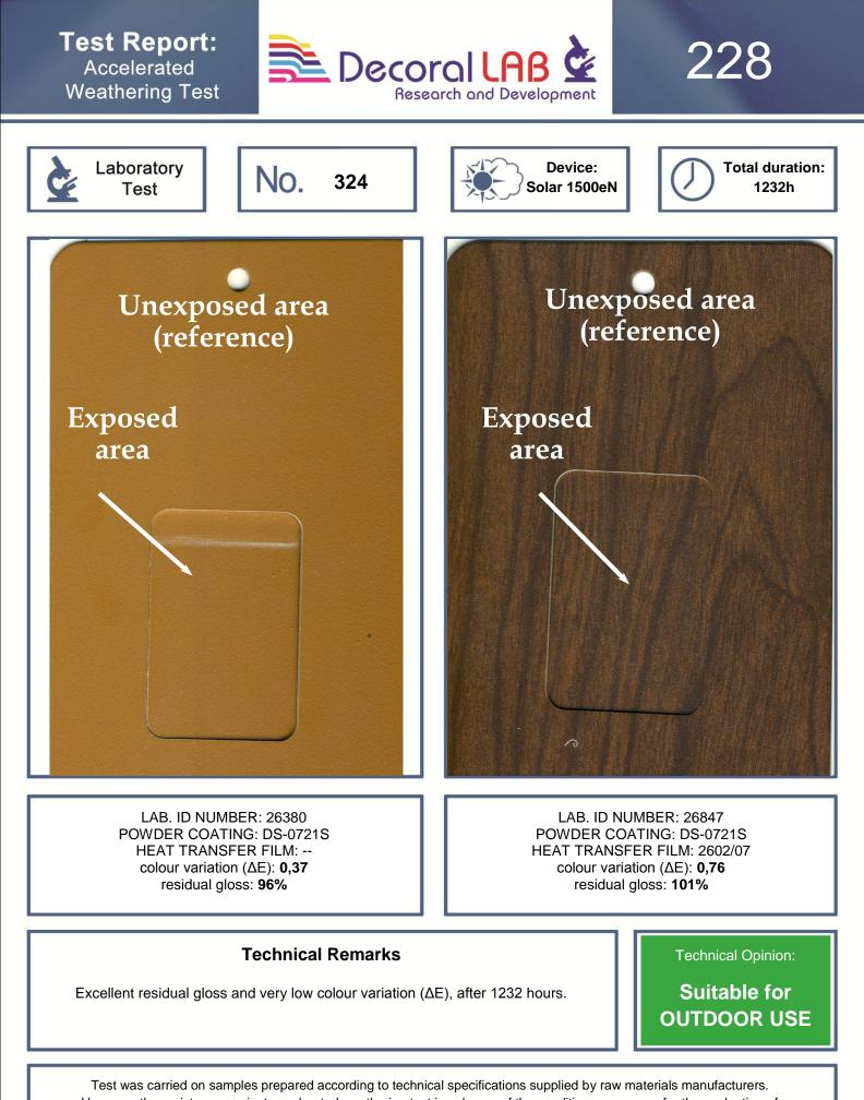
However, the resistance against accelerated weathering test is only one of the conditions necessary for the evaluation of the resistance of the finished product. For a final assessment see further analysis on natural exposure in Florida.
