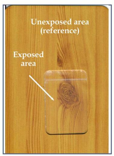
LAB. ID NUMBER: 26256 POWDER COATING: DS 1716 HEAT TRANSFER FILM: -colour variation (ΔΕ): 0,55 residual gloss: 60% LAB. ID NUMBER: 26287 POWDER COATING: DS 1716 HEAT TRANSFER FILM: 2103/01 colour variation (ΔΕ): **2,01** residual gloss: **71%**
