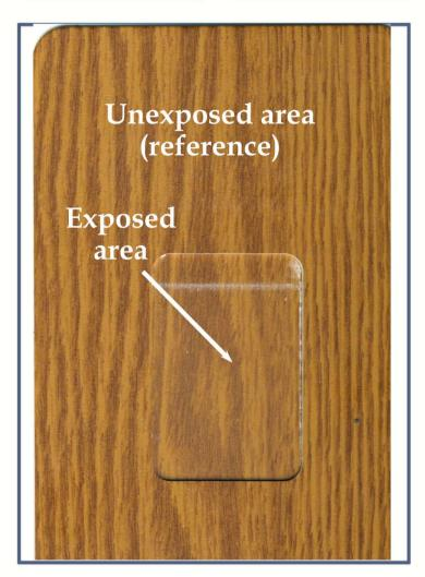
LAB. ID NUMBER: 26250 POWDER COATING: DS 739 HEAT TRANSFER FILM: --Colulor variation (ΔE): **0,32** residual gloss: **78%**  LAB. ID NUMBER: 26251 POWDER COATING: DS 739 HEAT TRANSFER FILM: 2513/02L Colulor variation (ΔΕ): **1,04** residual gloss: **66**%
