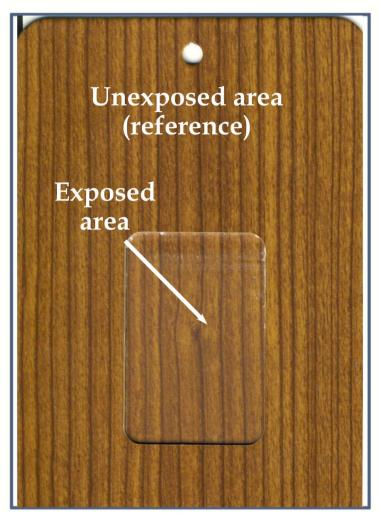
LAB. ID NUMBER: 26260 POWDER COATING: DS 755 HEAT TRANSFER FILM: --Colulor variation (ΔE): **0,45** residual gloss: **81%**  LAB. ID NUMBER: 26261 POWDER COATING: DS 755 HEAT TRANSFER FILM: 1402/02L Colulor variation (ΔΕ): **1,35** residual gloss: **72**%
