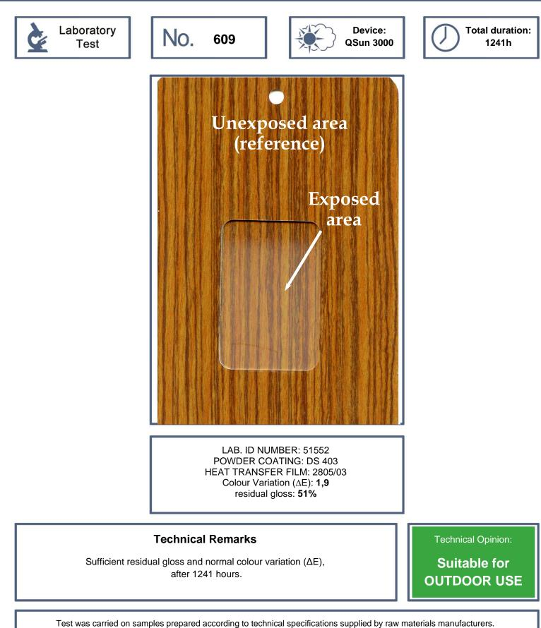
Test was carried on samples prepared according to technical specifications supplied by raw materials manufacturers. However, the resistance against accelerated weathering test is only one of the conditions necessary for the evaluation of the resistance of the finished product. For a final assessment see further analysis on natural exposure in Florida.
