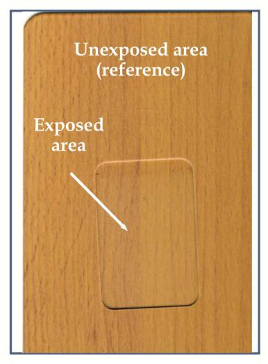
LAB. ID NUMBER: 26309 POWDER COATING: DS 402 HEAT TRANSFER FILM: -colour variation (ΔΕ): **0,28** residual gloss: **86%**  LAB. ID NUMBER: 26310 POWDER COATING: DS 402 HEAT TRANSFER FILM: 1603/02L colour variation (ΔΕ): **2,38** residual gloss: **88%**
