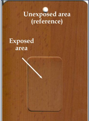
LAB. ID NUMBER: 26301 POWDER COATING: DS 453 HEAT TRANSFER FILM: -colour variation (ΔΕ): **0,10** residual gloss: **63**% LAB. ID NUMBER: 26302 POWDER COATING: DS 453 HEAT TRANSFER FILM: 1603/02L colour variation (ΔΕ): **0,78** residual gloss: **60%**
