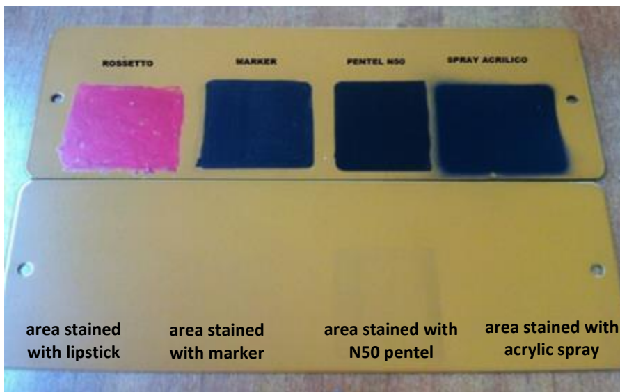
ABOVE: Soiled panel painted with DS-0821SA.
