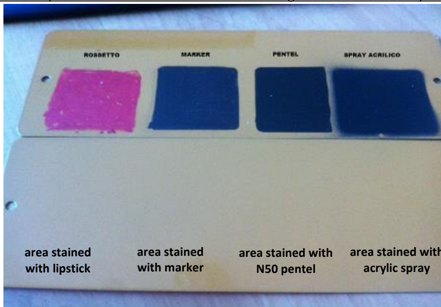
ABOVE: Soiled panel painted with DS-0821SA.
