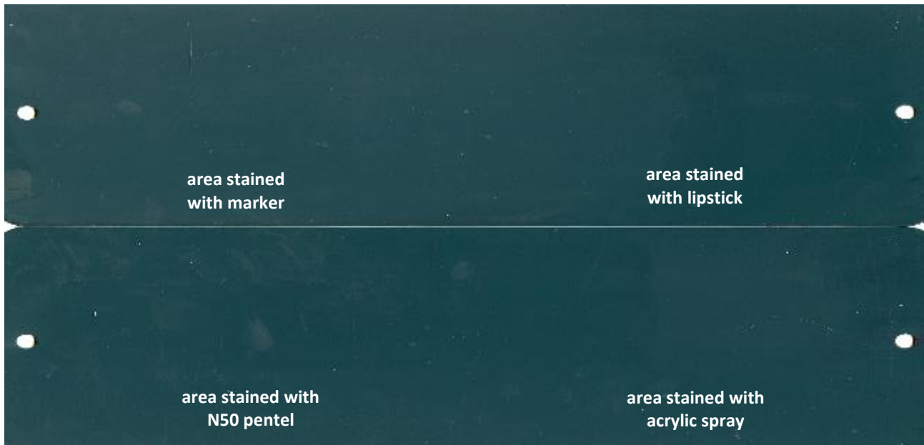
ABOVE: Painted Sample Panel after the cleaning with a mixture of Etasol/MEK 70:30
