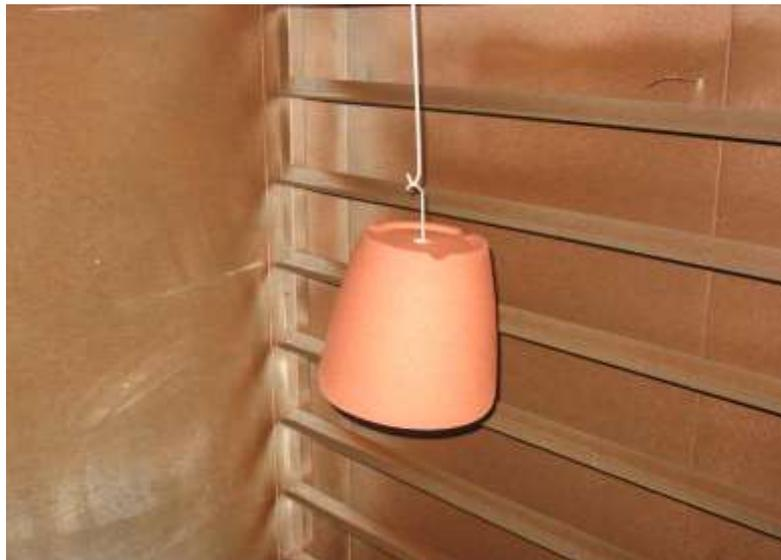
Picture 3: the sample inside the oven with its support, to complete the curing
