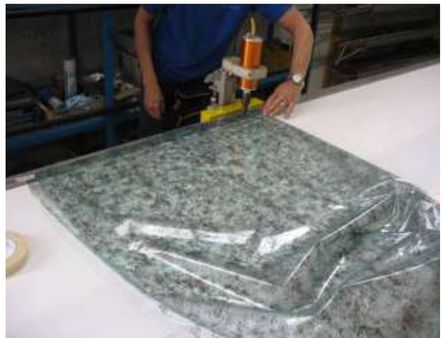
Picture 6: one remaining side is closed, forming a bag
