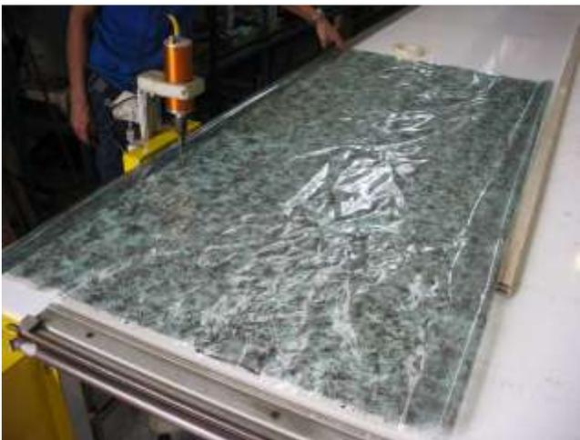
Picture 5: two sides of the portion of film are joined together
