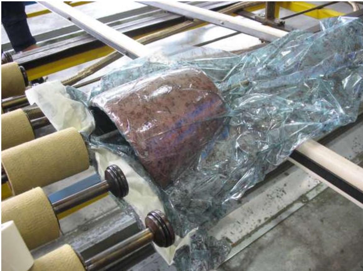
Picture 9: the bag containing the object is closed on the suction head (on the left), then vacuum is made
