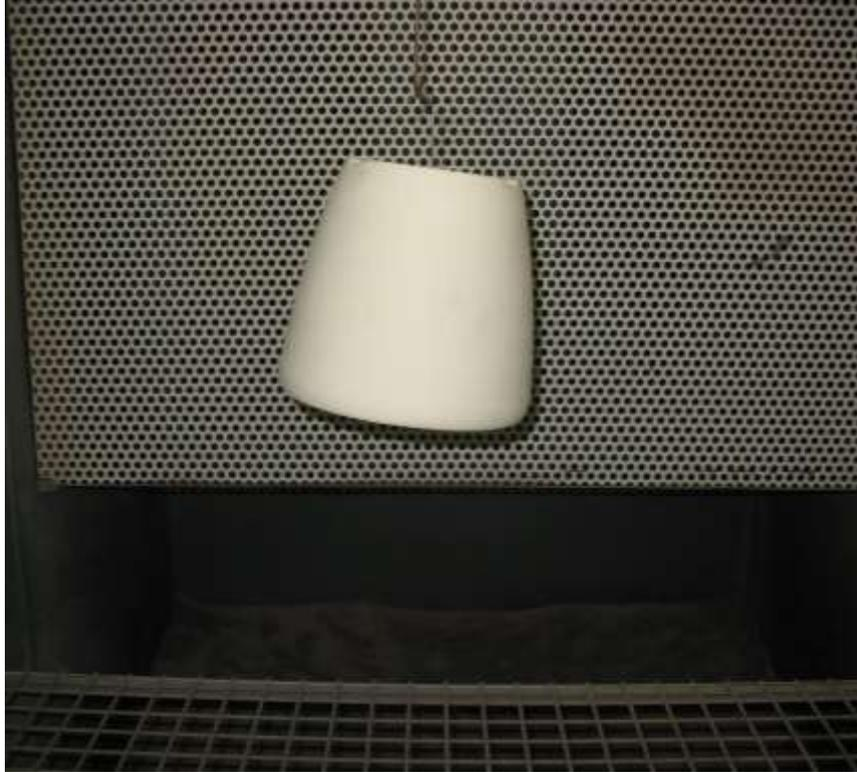
Picture 1: preparation of the sample on a hook, in order to move it without touching it
