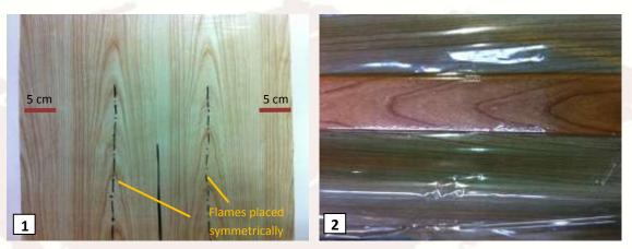
Select a portion of the film that comprises two flames, symmetrically placed to one another; then, cut the film on the borders, leaving 5 cm on the outer side of each flame.
