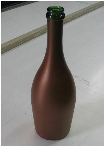
Picture 12: powder-coated sample
