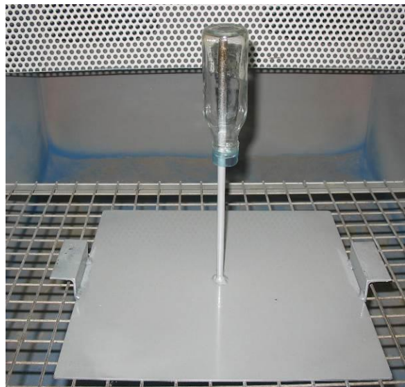
Picture 6: preparation on the support for the powder-coating
