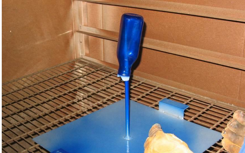
Picture 9: the sample inside the oven on its support, to complete the curing
