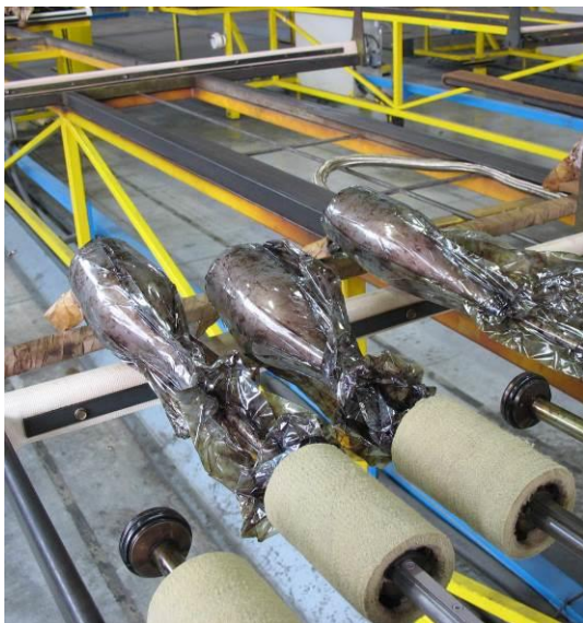
Picture 18: glass bottles just after the sublimation in the oven
