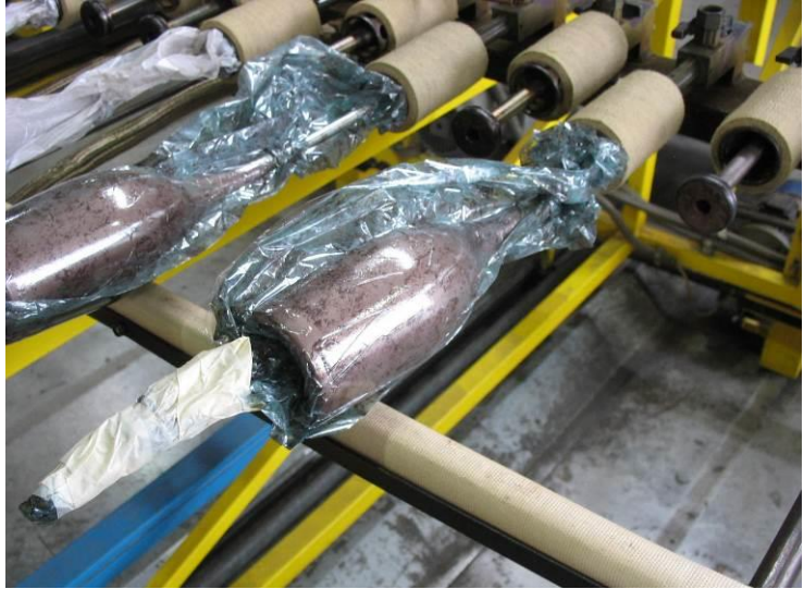
Picture 17: sample in its bag, closed on the “suction heads”
