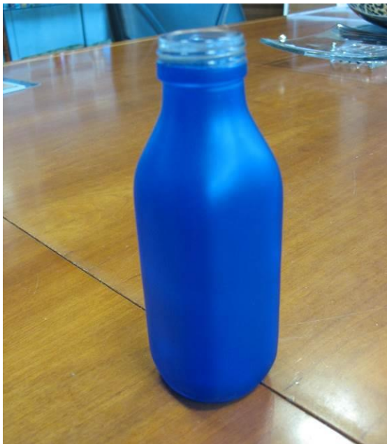
Picture 10 and 11: the sample powder-coated with Glass-003
