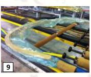
Vaccum using two heads (or one head, closing the other end)
