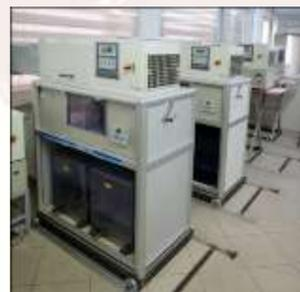
Accelerated Weathering Test devices
