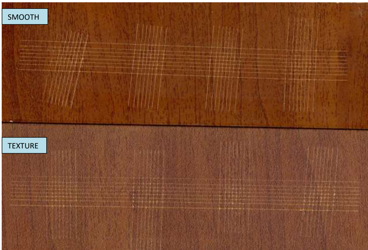
Figure 7: Result of the adhesion test on a decorated MDF sample
