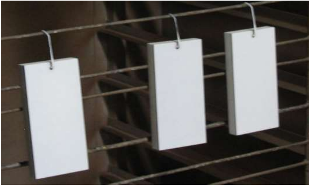
Figure 5: Sample put back into the oven at 160° for the curing cycle
