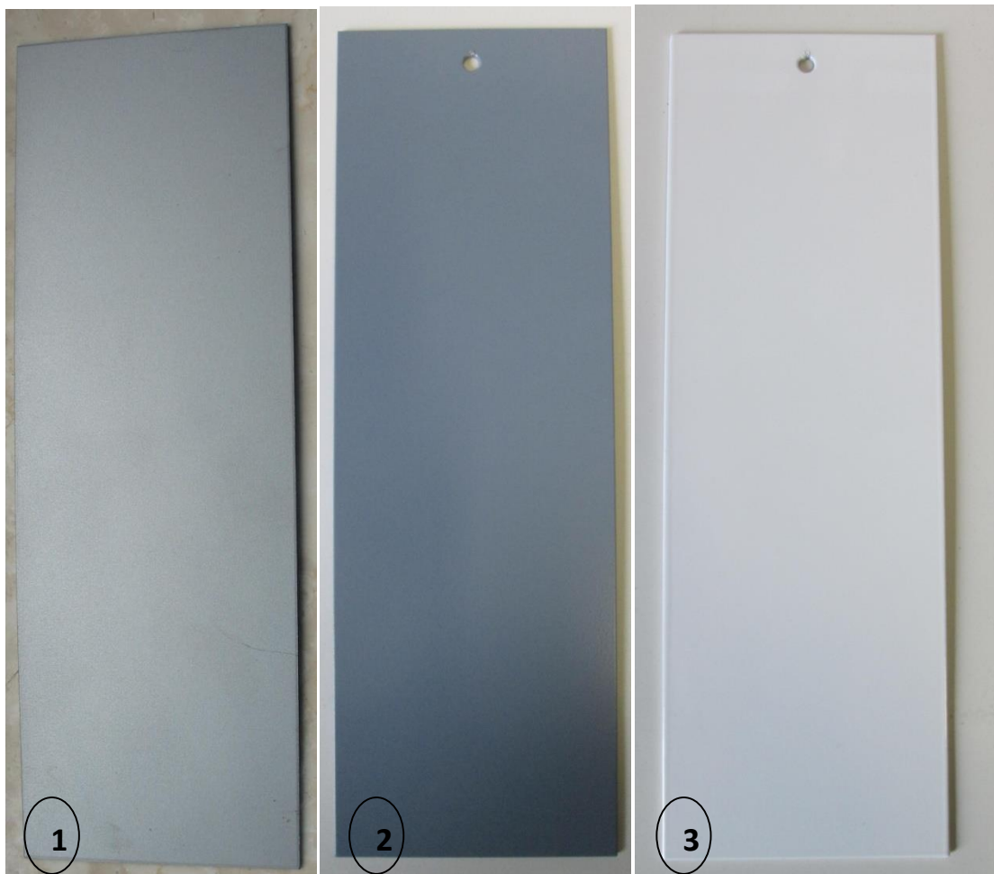
Picture 1: Iron alloy panel after sandblasting.
