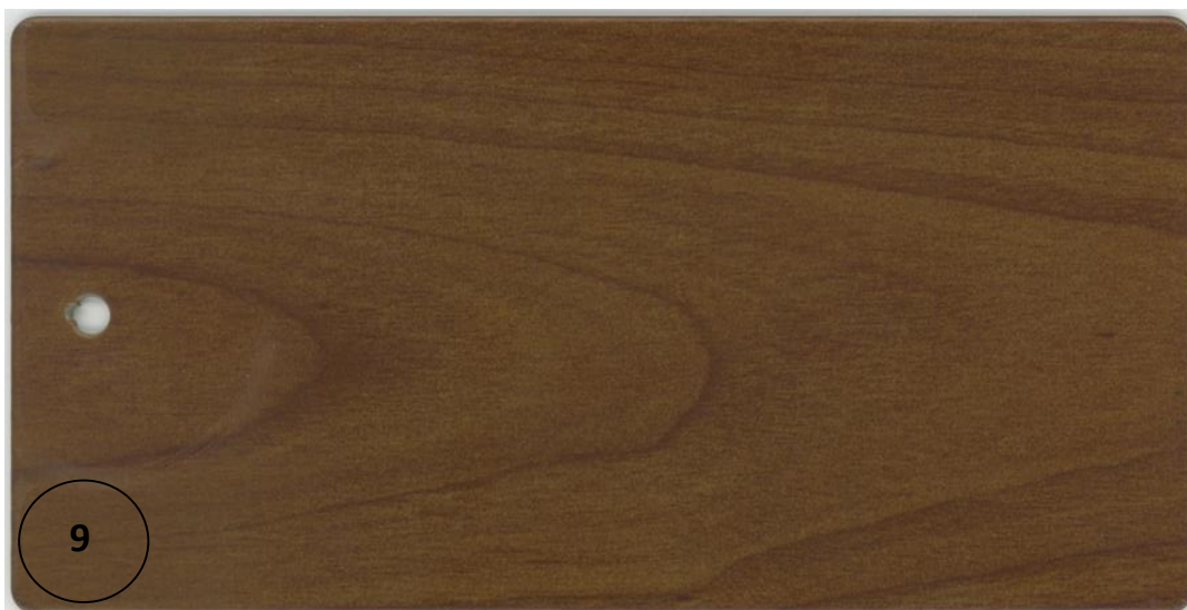
Picture 9: Sandblasted, overpainted and decorated sample panel with Ironsafe-01 after the resistance test.
