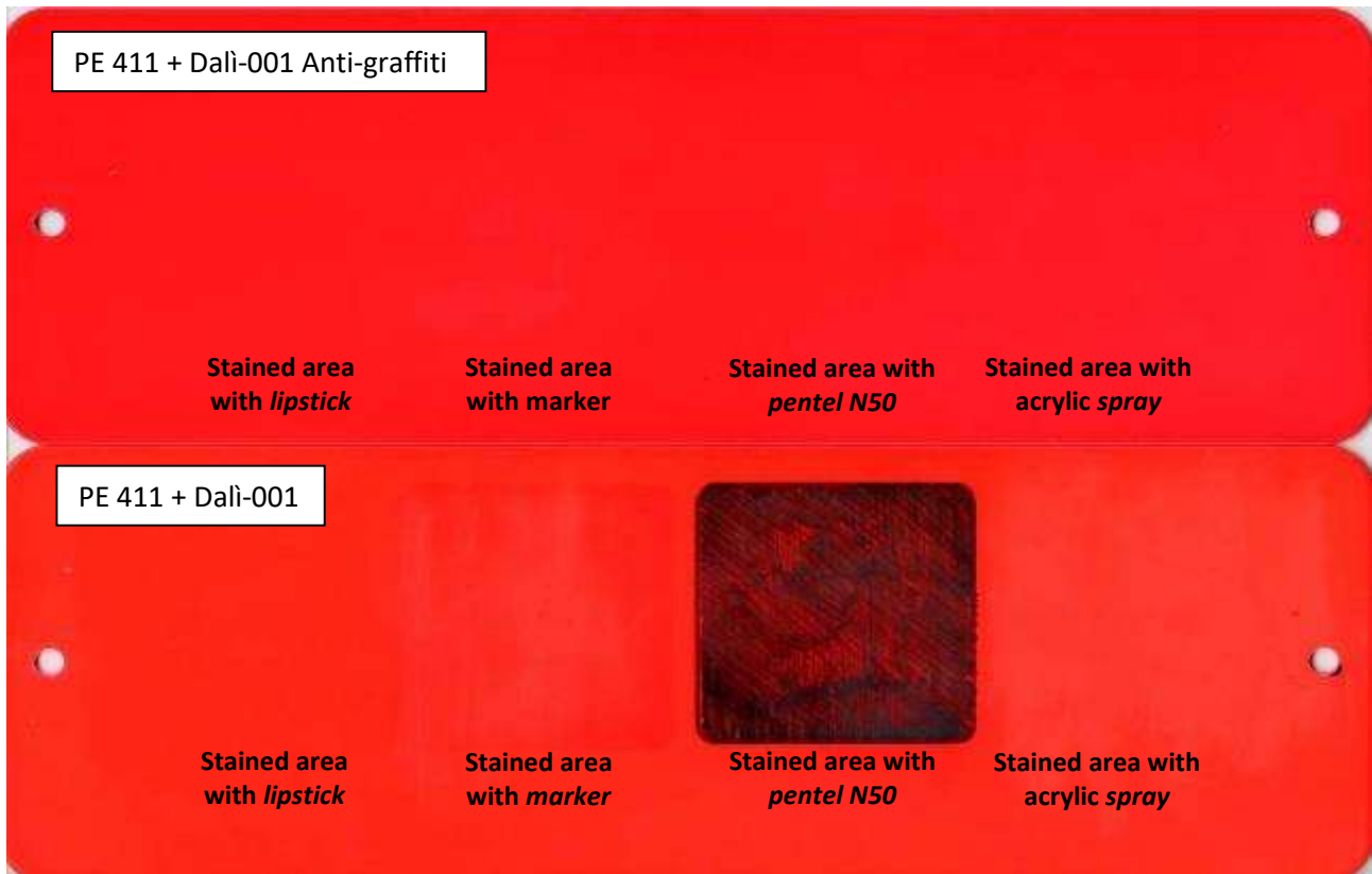
Figure 5: Comparative Antigraffiti test on different sample of powder coating
