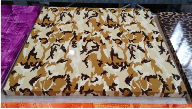
Flat surface double coated and decorated with heat-transfer film on paper carrier 6010/56 C
