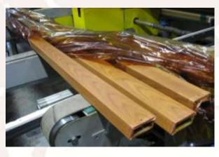
The bag is easily removed: the decorated profiles show no stain and the wood effect has been perfectly transferred.
