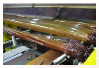
Profiles coming out of the oven: the exhausted film is removed from their surface with an air jet in the bag.
