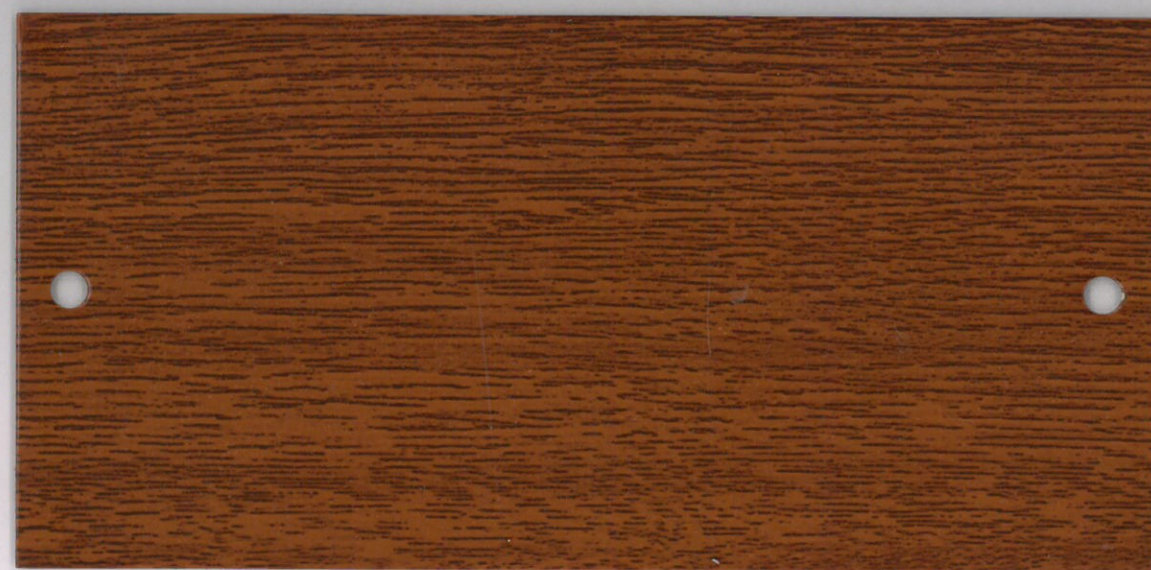
Powder Coating: DS 742 + Heat Transfer Film: 2309/03
