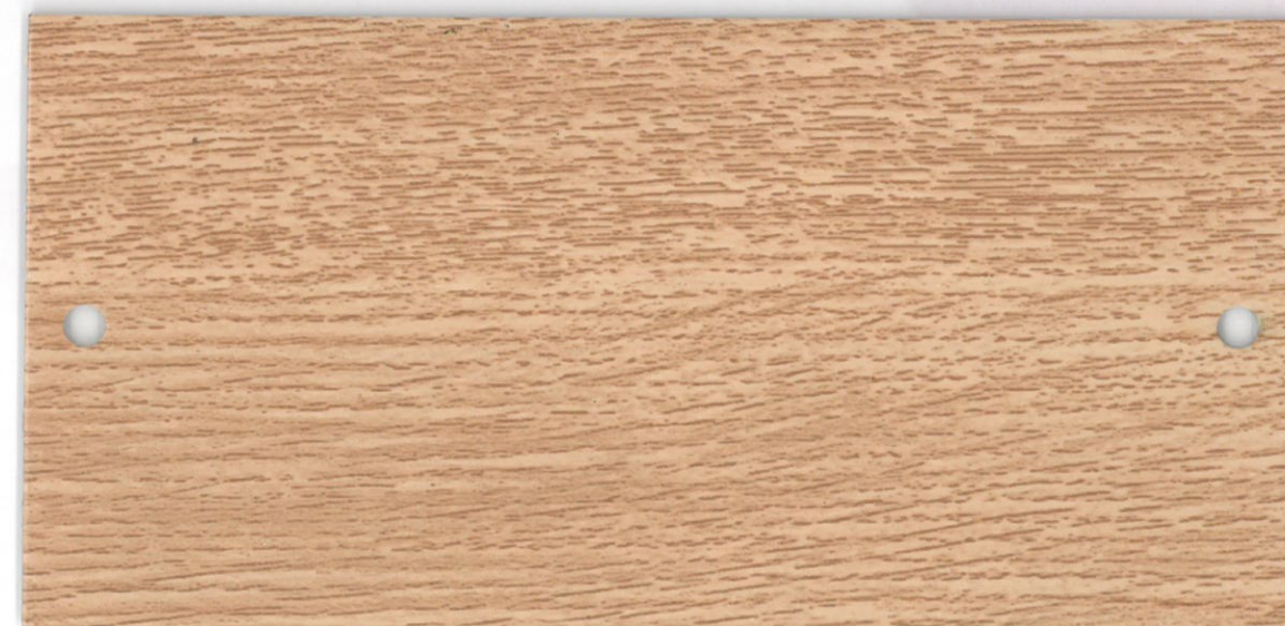
Powder Coating: DS 746 + Heat Transfer Film: 2309/06
