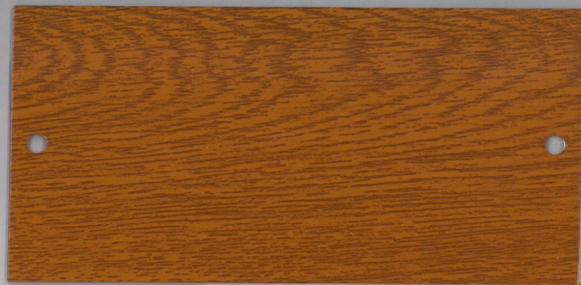
Powder Coating: DS 725 + Heat Transfer Film: 2309/02
