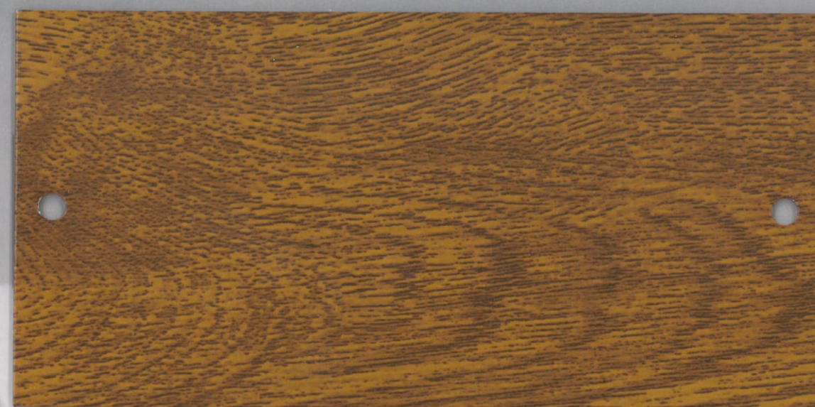
Powder Coating: DS 730 + Heat Transfer Film: 2309/02
