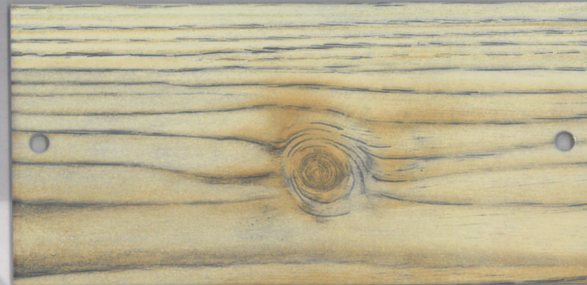
Powder Coating: DS 405 + Heat Transfer Film: 2112/01
