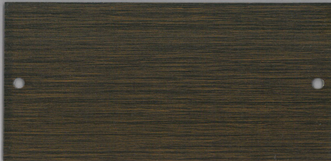
Powder Coating: DS 775 + Heat Transfer Film: 2502/12
