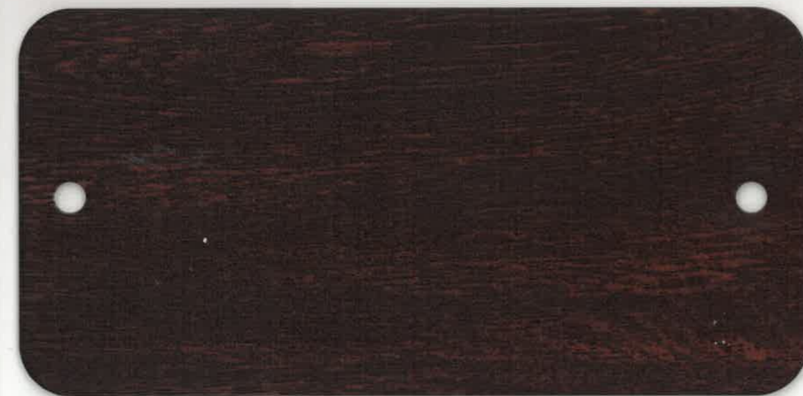
Powder Coating: DS 706 + Heat Transfer Film: 2302/03
