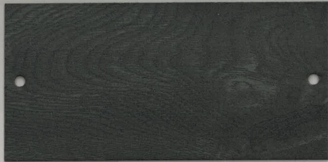
Powder Coating: DS 770 + Heat Transfer Film:2302/03
