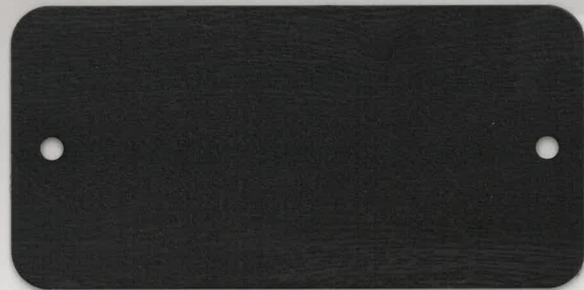
Powder Coating: DS 757 + Heat Transfer Film: 2302/03
