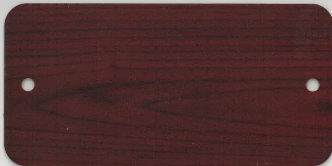
Powder Coating: DS 794 + Heat Transfer Film: 1109/03
