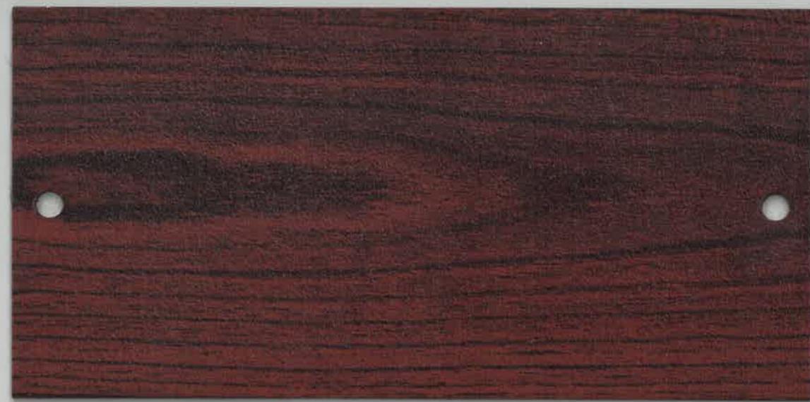
Powder Coating: DS 706 + Heat Transfer Film: 1413/03
