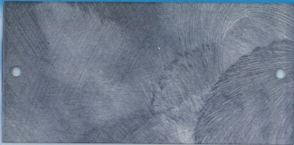
Powder Coating: ICE TOUCH-001 + Heat Transfer film: 5007/01
