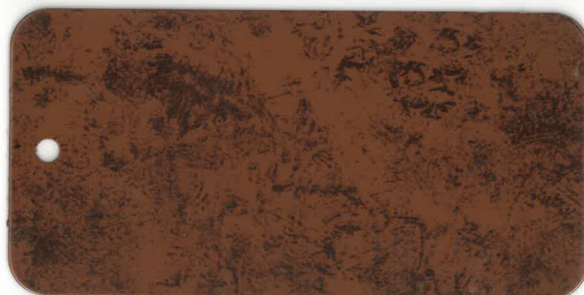
Powder Coating: 9B-036-A004 + Heat Transfer Film: 6052/01L
