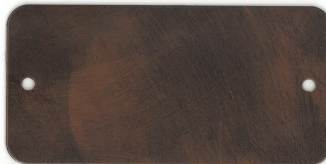
Powder Coating: 9C-036-A004 + Heat Transfer Film: 5007/01L
