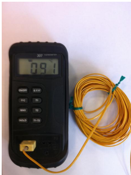
Picture 2: temperature monitoring probe
