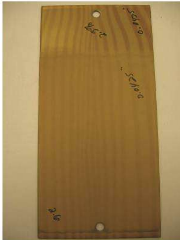
Photo No. 3 60 Month Weathering Sample - South Florida Exposure
