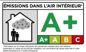
The product was assigned a VOC emission class without taking into account the measurement uncertainty associated with the result. As specified in French Decree no. 2011-321 of March 23, 2011, correct assignment of the VOC emission class is the sole responsibility of the party responsible for distribution of the product in the French market.
