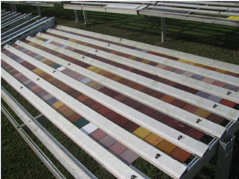
Picture 3: Florida Natural Exposure, test samples.
