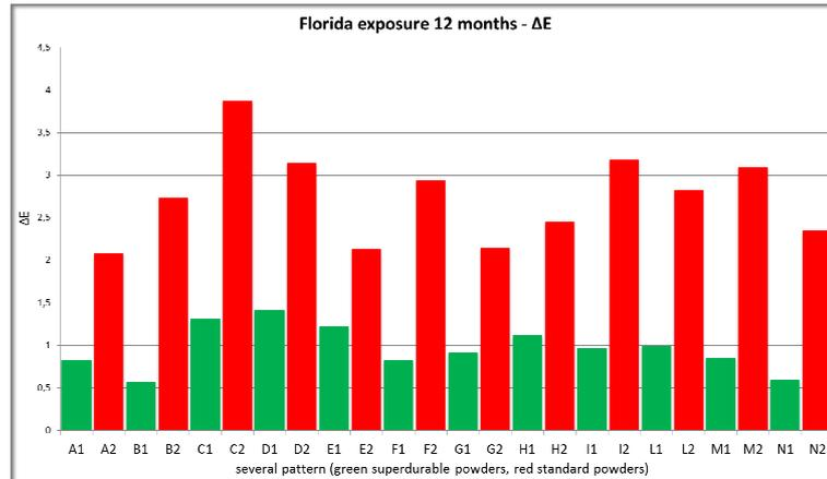
Picture 7: 12 months NET in Florida: comparison between the values of measured  $\Delta E$ , green samples representing superdurable products.
