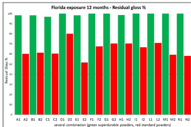
Picture 6: 12 months NET in Florida, comparison between the values of percentage of residual gloss, green samples representing superdurable products.
