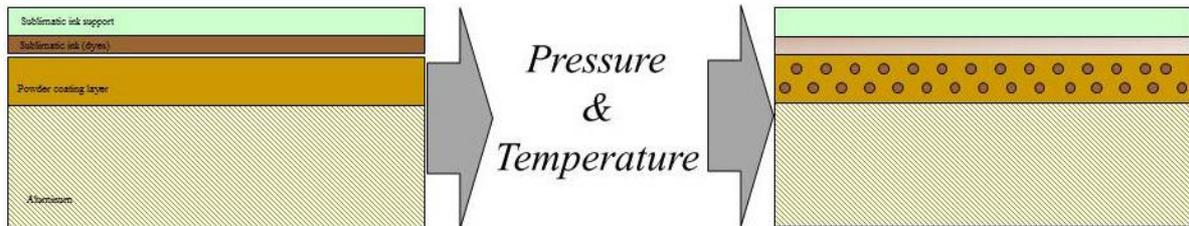
Picture 1: process of sublimation, ink transfer in the pre-coated layer of coating.
