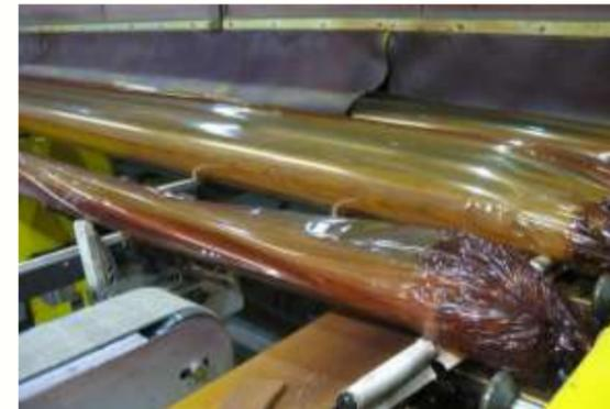
Profiles coming out of the oven: the exhausted film is removed from their surface with an air jet in the bag.
