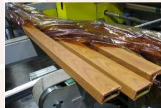
The bag is easily removed: the decorated profiles show no stain and the wood effect has been perfectly transferred.
