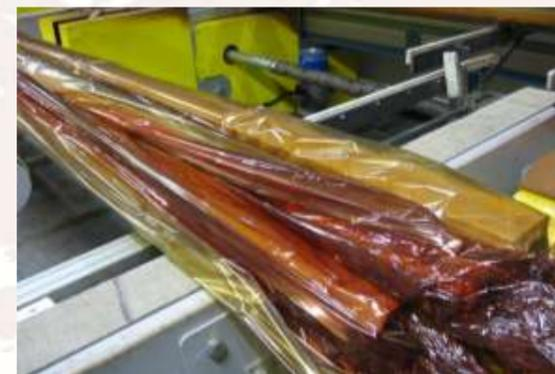
Profiles are piled on each other still closed in their bags. The inks in excess do not represent a problem for the decorated object, since they have been absorbed into the layer of *primer* of the carrier *L*.
